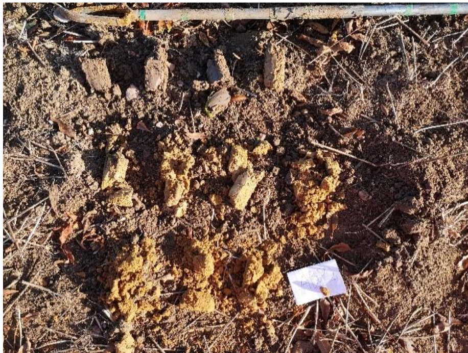
Figure 4.3: Soil Type 3 – Calcareous loam over loamy sand or sand Source: Mott MacDonald, November 2021
